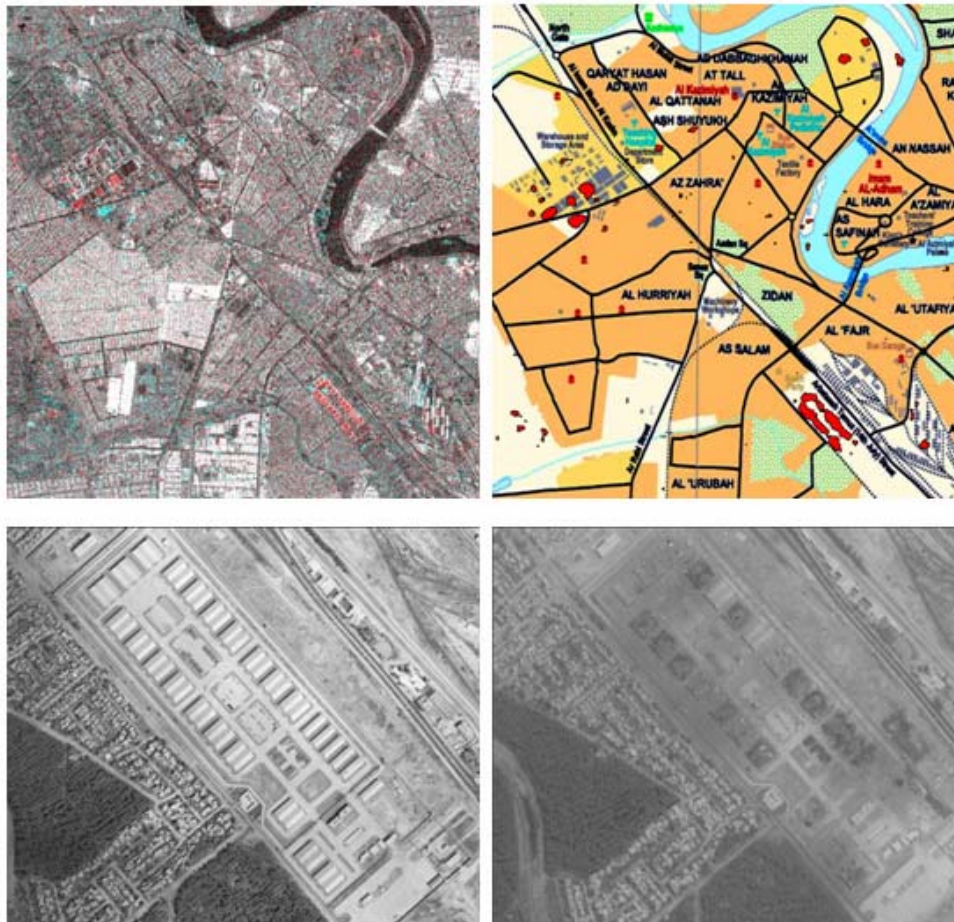
Figure 5. Top-left: Radarsat colour composite. Top-right: corresponding map with changes (red) in overlay. Bottom-right: Quickbird before destruction. Bottom-left: Quickbird after destruction.
